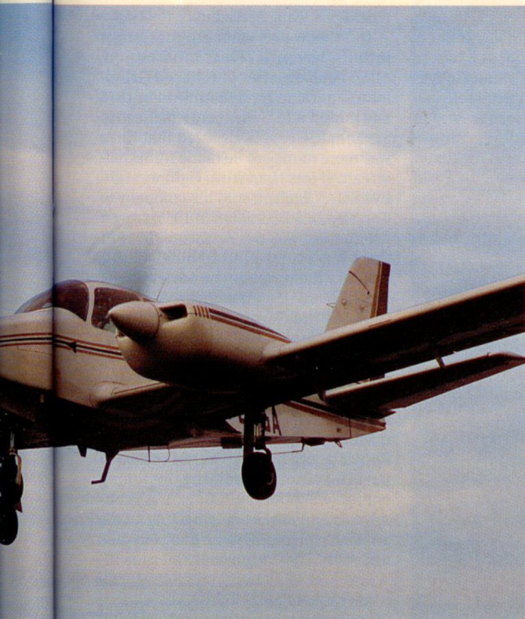
The Cougar's distinctive, pointed nose offers excellent forward visibility; the pilot can barely see it. Visible under the nose on the right side is an antenna for relaying television signals. This Cougar earns its pay loitering for hours over championship bicycle races.
